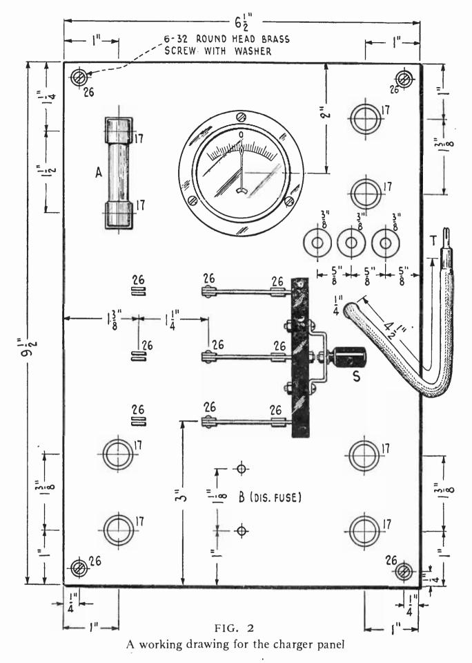
the commercial rectifier is cased, and which absorbs a considerable amount of energy which would otherwise be spent as useful charging current. If the parts are removed from the metal box, and simply connected together on a baseheard, the charging rate will compating he in the rectifier circuit. The meter reads both charge and discharge up to fifteen amperes, and is the type mounted on automobile instrument boards.
