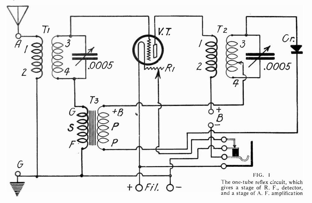
operate a loud speaker over distances about equal to those it is possible to hear with the telephones on an ordinary crystal receiver. When used with a headset it is capable of very long distance reception, extremely sharp tuning, and exceptionally clear reproduction of speech and music.
