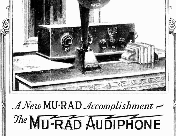
The super-sensitive mica diaphragm produces sound by the contraction and expansion of an actuating contact, just as the vocal cords produce the voice.
