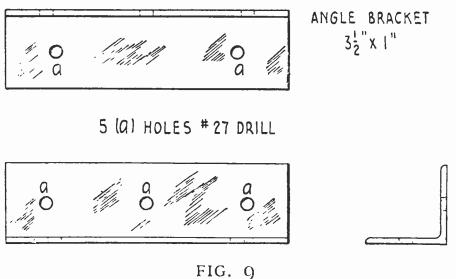
This is the bracket (half actual size) that fastens the sub-panel to the main panel
