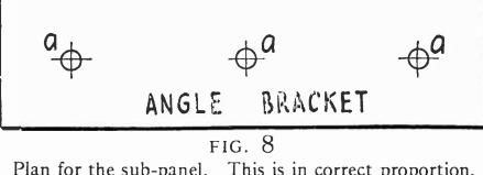
Plan for the sub-panel. This is in correct proportion, but less than actual size  $(\frac{11}{14})$ . For *a* holes, use No. 27 drill; for *b* holes, use No. 52 drill
