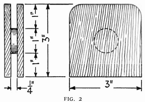
This special transformer is used to couple the last R. F. tube to Detector Tube No. 2 in Fig. 1, and provides a sharp resonant point for the radio-frequency circuit. The walls of this transformer may be made of bakelite or hard rubber. The primary is wound with 200 turns of No. 29 D. S. C. and is separated from the secondary, which has 1500 turns of No. 36 D. S. C., by several layers of empire cloth
