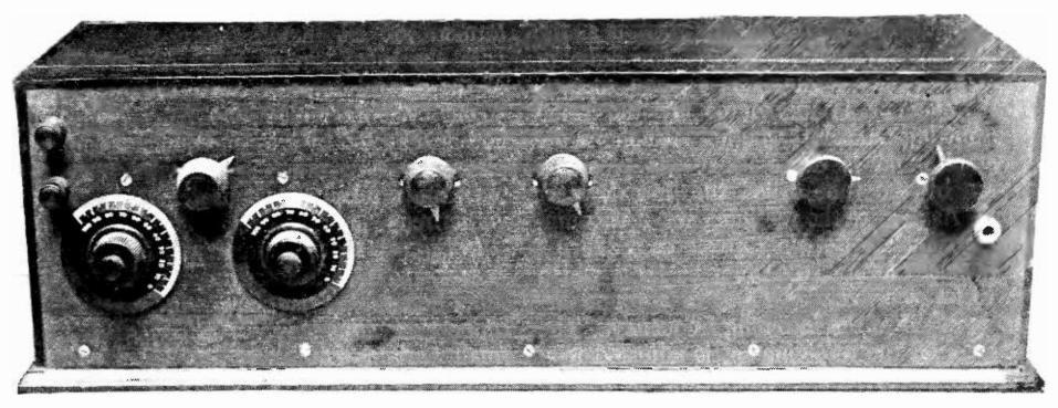
MR. ELTZ'S SEVEN-TUBE SUPER-HETERODYNE It has but two tuning controls. The simplicity of operation of a set of this type is sure to make it increasingly popular
